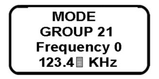
Press ENTER to lock in the (example) Frequency 123.45 Khz
